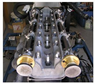
Variable Valve Timing head installed in the engine in the test stand
